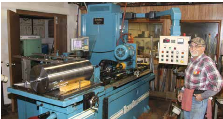
Above : A gun drill at Land Specialties Manufacturing.
