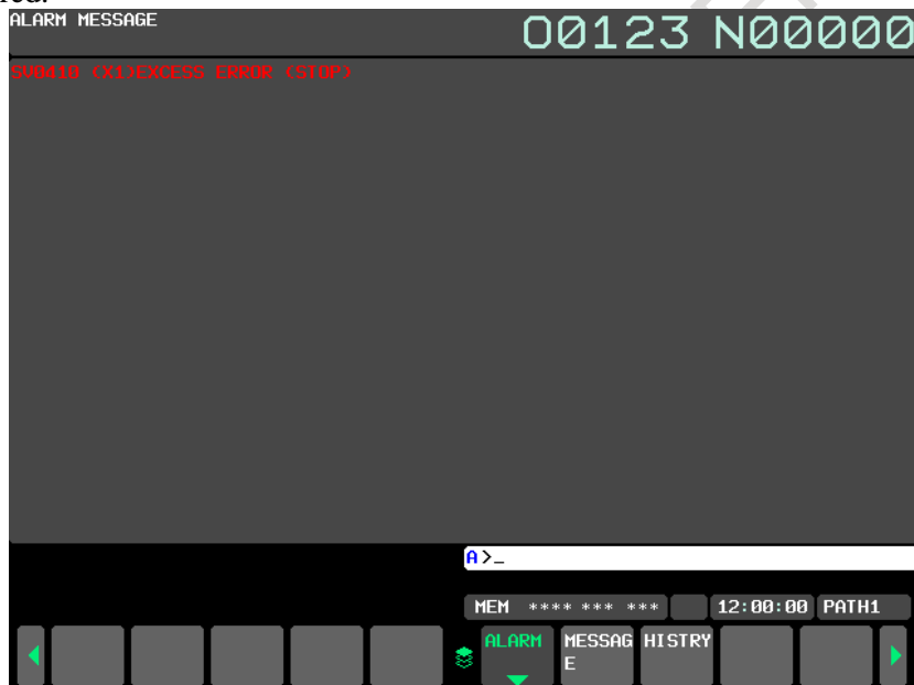
Fig.18.4.1 (a) Alarm message screen (10.4-inch display unit)
