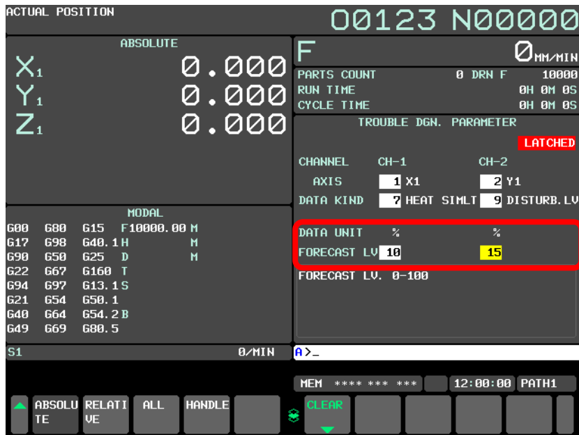
Fig.18.4.6 (b) Setting of trouble forecast level on the trouble diagnosis parameter screen
