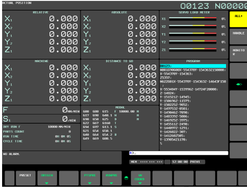
Fig. 13.1.23 (c) Current position display of 15 inch (overall)
