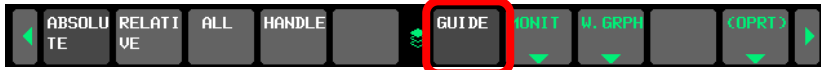
Fig.18.4.1 (j) Soft key to select trouble diagnosis guidance screen (10.4-inch display unit)
