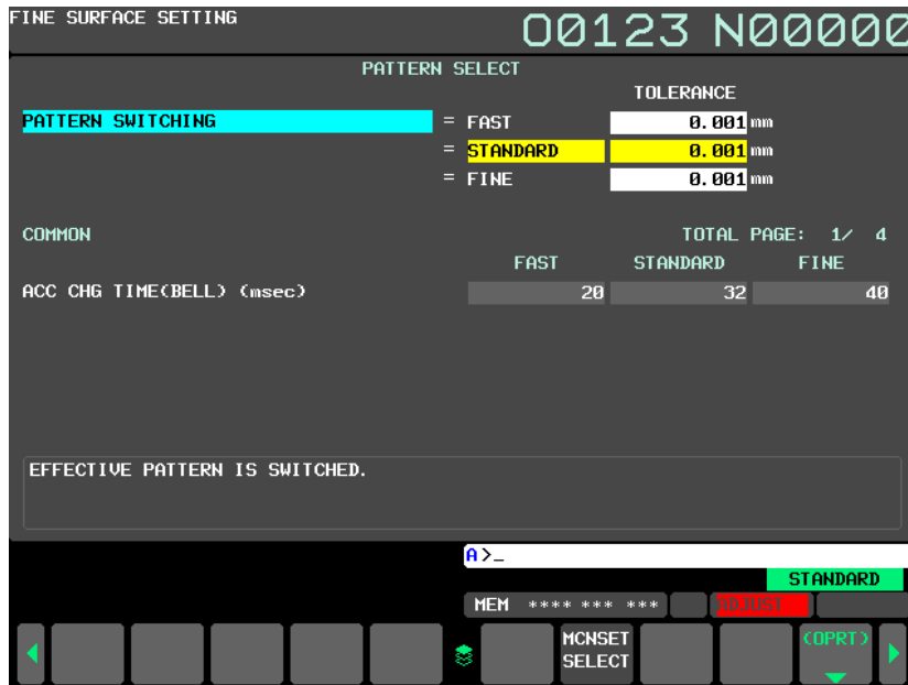
Fig. F.3 (i) Display setting values of setting pattern (common)(pattern select screen)
