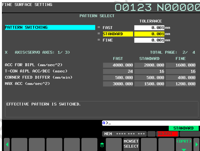
Fig. F.3 (j) Display setting values of setting pattern (each axes)(pattern select screen)
