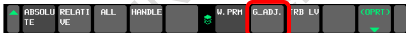
Fig.18.4.1 (h) Soft key to select trouble diagnosis graphic screen (10.4-inch display unit)
