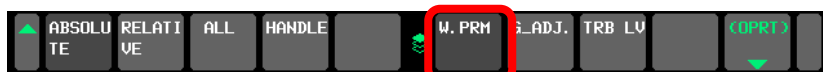
Fig.18.4.1 (f) Soft key to select trouble diagnosis parameter screen (10.4-inch display unit)
