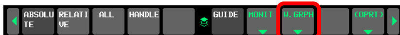
Fig.18.4.1 (e) Soft key to select trouble diagnosis graphic screen (10.4-inch display unit)
