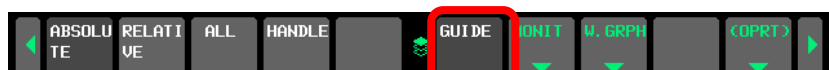
Fig.18.4.1 (b) Soft key to select trouble diagnosis guidance screen (10.4-inch display unit)
